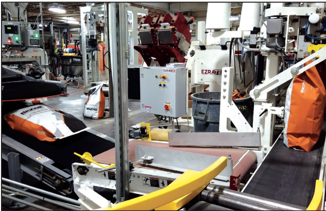
The conveyance line has a bag kicker, flattener and an innovative optional bypass line for buckets.
