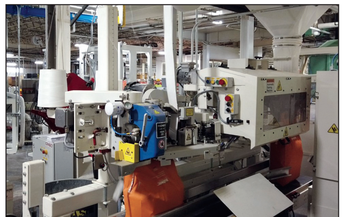
Automatic product filling, moving to laser printing, then moving to sewing on the conveyor line.
