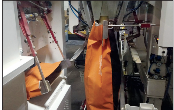
The auto bag placer opens the top of the bag and places it under the filling spout.
