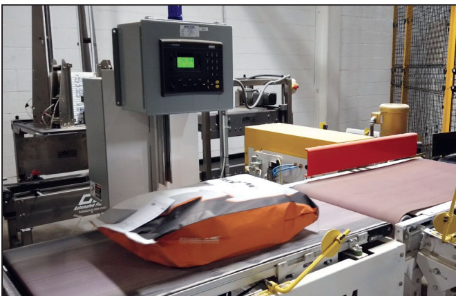
Check weigh station in conveyor line with a reject conveyor for quality control.
