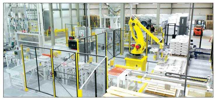
Magnum Systems' total system solution for moving and bagging mineral products in 50 lb and 1,000 - 2,000 lb bulk bags from start to finish at The Quartz Corporation.
