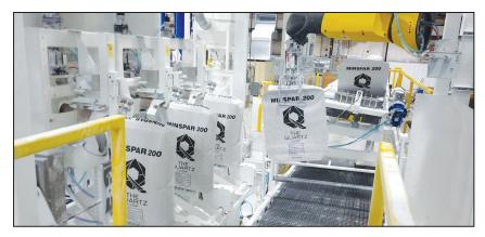
Three Model A Valve Bag Fillers with Robotic Bag Placing for packing of 50 lb bags.
