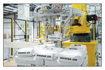
Model TRP-3000 robotic palletizing 50 lb bags to be shrink-wrapped for delivery.
