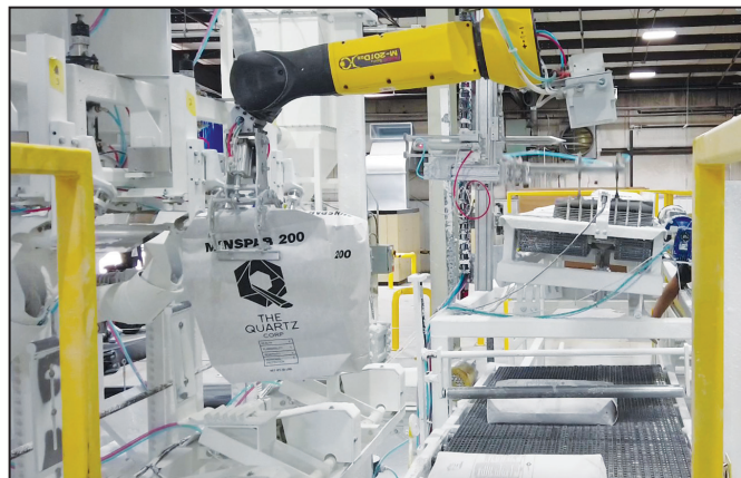
Model TRV-1000 robot placing 50 lb. bags for filling and conveying.
