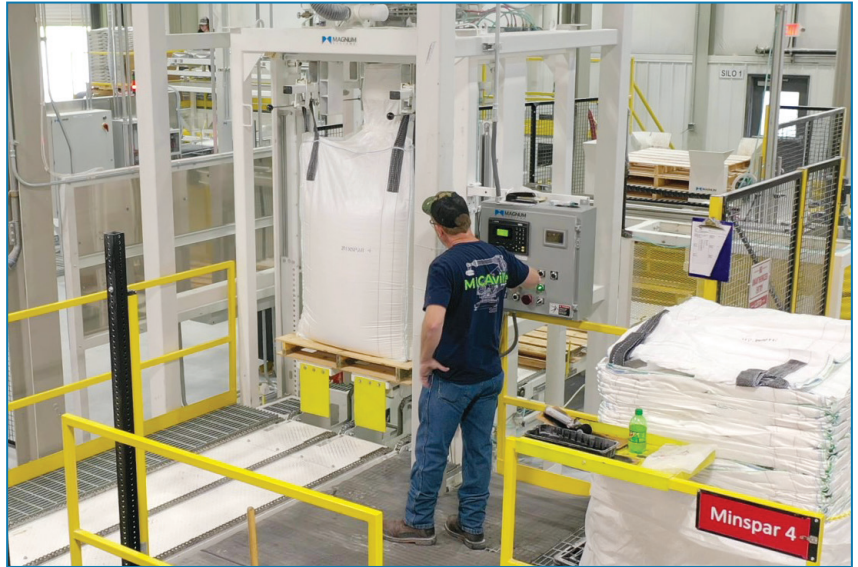
Model IBC-3000 filling and weighing 1,000 and 2,000 lb. bulk bags at The Quartz Corporation.
