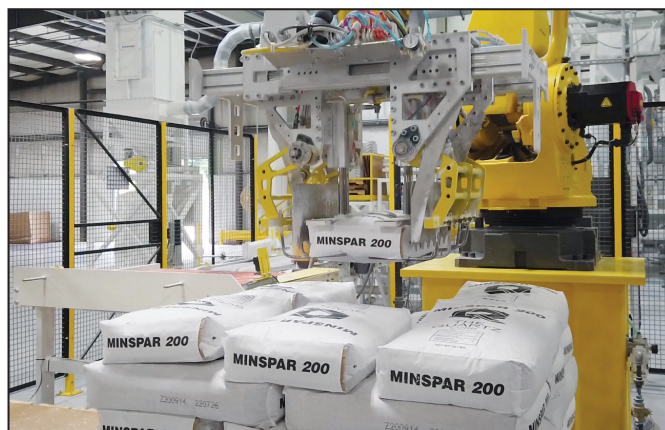
Model TRP-3000 robotic palletizing 50 lb. bags to be shrink wrapped for delivery.
