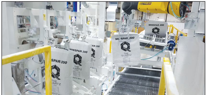
Three Model A Valve Bag Fillers with Robotic Bag Placing for packing of 50 lb. bags.
