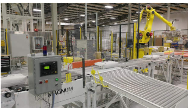
Figure 2. Automated system example moving 50 lb bags on belt conveyors, roller conveyors, and robotics for palletisation of material.
