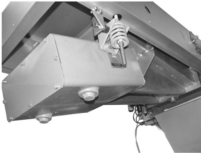
Figure 1-3. Vibratory Feeder
