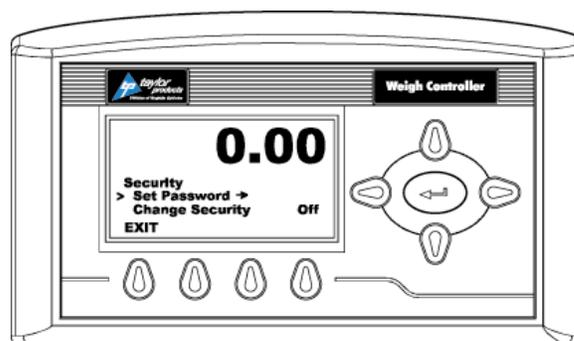
Figure 3-7. Placing The Cursor In Front Of Set Password
