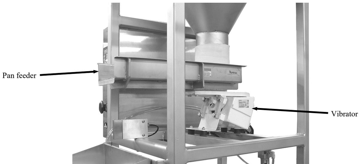
Figure 1-3. Vibrator Pan Feeder
