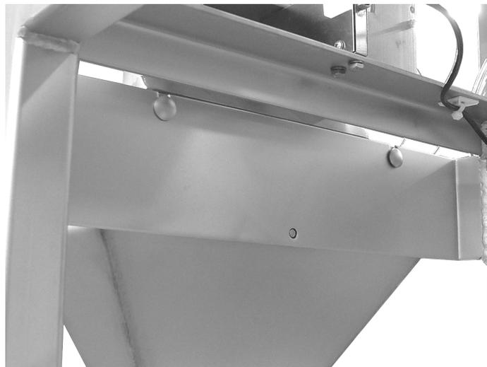
**Figure 7-12.** Discharge Spout Pins Properly Secured In The Mounting Bracket
