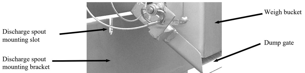
**Figure 3-5.** Discharge Spout Mounting Bracket
