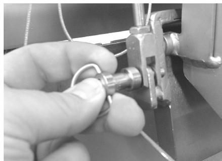
**Figure 7-5.** Removing the Lower Gate Cylinder Retaining Pin
