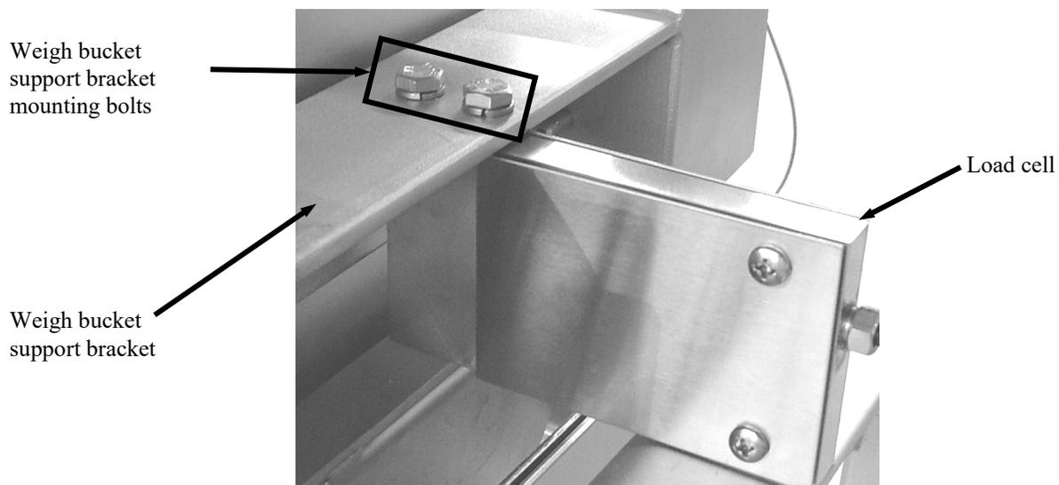
Figure 3-1. Weigh Bucket Support Bracket Mount
