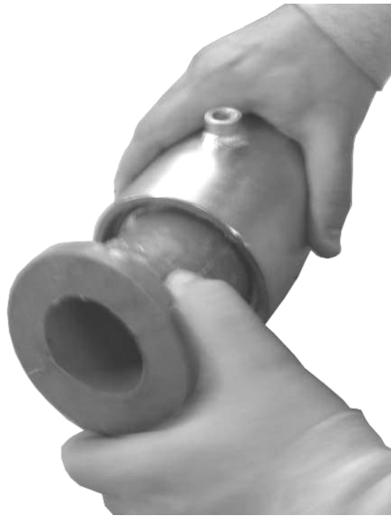
Figure 7-18. Remove The Pinch Valve Liner From The Housing
