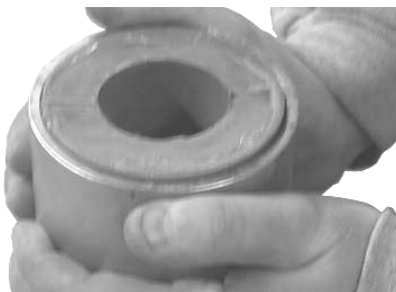
Figure 7-22. Invert the Housing And Press Down
