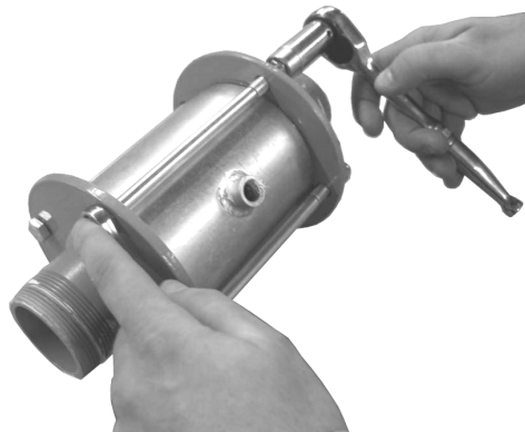
Figure 7-24. Install The Bolts And Nuts
