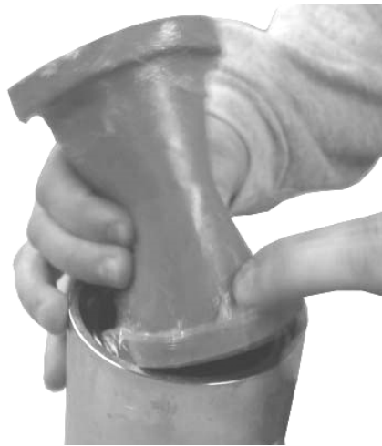
Figure 7-20. Slide The Pinch Valve Liner Into The Housing
