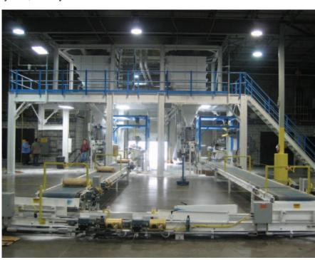
The two parallel packaging lines consistently fill up to 24 bags per minute, exceeding the company's original packaging rate requirements.
