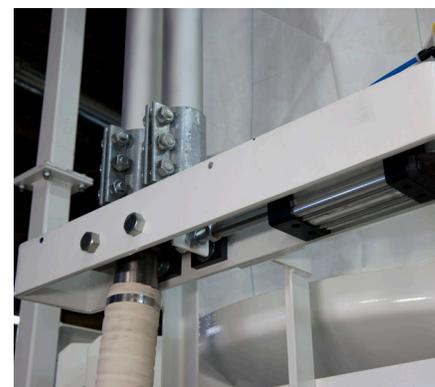
**Magnum Systems Slide Diverter Valve (SDV) is for use in pneumatic conveying of dry materials, wherever the flow of product must change from one line to another.**
