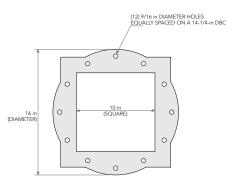
NOTE: AIRLOCK FLANGES ARE PROVIDED WITH BOTH SQUARE AND ROUND FLANGE PATTERN DRILLING.
