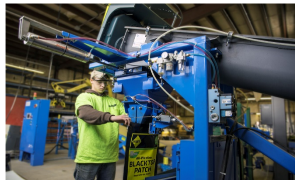
Operator Placing Bag on Gross Weigh Scale
