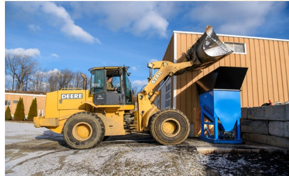
End Loader & Inlet Hopper
