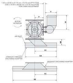
NOTE: CENTER MOTOR MOUNTING HOLE IS NOT ALWAYS IN CENTER OF CYLINDER HOUSING (FT7, FT11, FT14, FT18) SEE DIMENSION  $\bf Q$  FOR OFFSET DISTANCE
