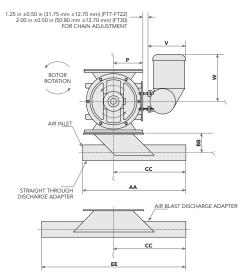
NOTE: CENTER MOTOR MOUNTING HOLE IS NOT ALWAYS IN CENTER OF CYLINDER HOUSING (FTZ, FT11, FT14, FT18) SEE DIMENSION  $\bf Q$  FOR OFFSET DISTANCE
