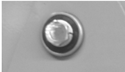
Figure 7-8. Shut Off Gate Mounting Screw Ground Off Smooth
