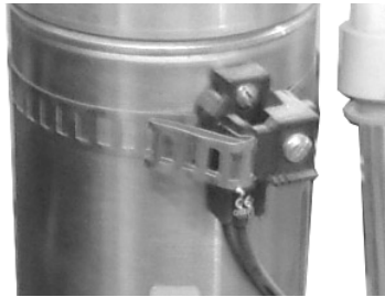
Figure 39 – Band Clamp Type Proximity Switch Installation
