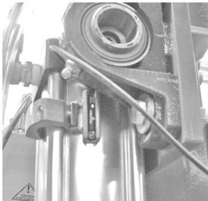
Figure 8 – Proximity Switch (Switch Is Made – LED On)
