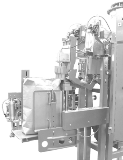
Figure 20 – Anvil And Horn Pinching The Fill Valve
