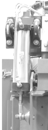
Figure 37 – Horn Cylinder (1 of 2 shown)
