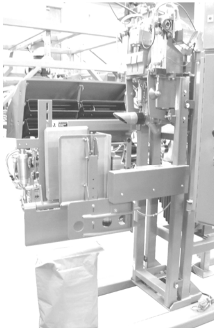
Figure 22 – Bag Chair In Down Position, Bag Has Dropped
