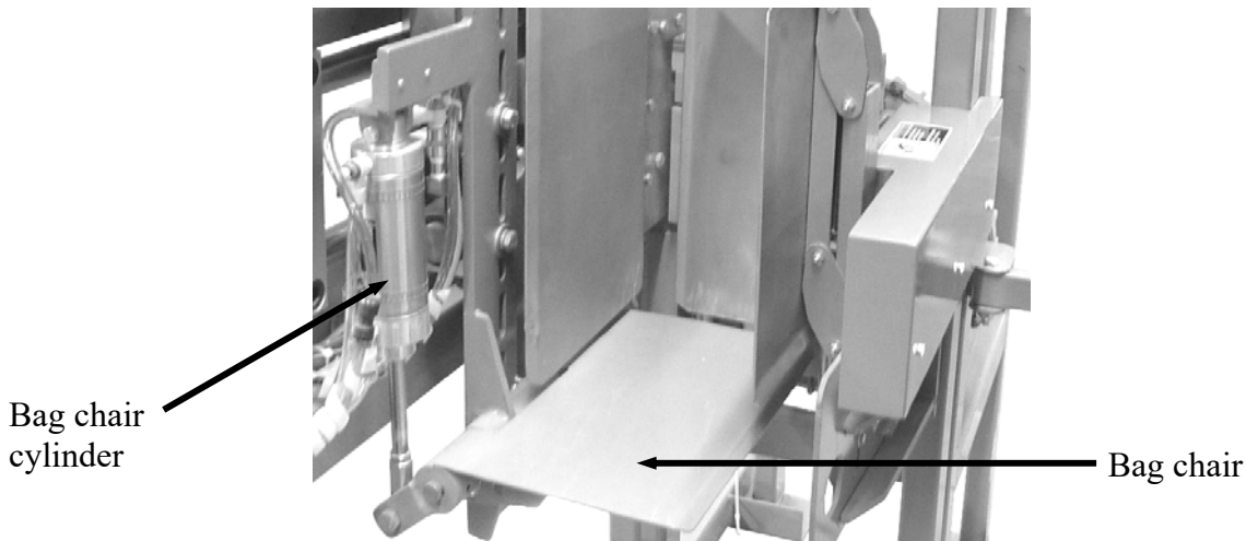
Figure 2 – Bag Chair and Pneumatic Cylinder (Shown in the Up Position)
