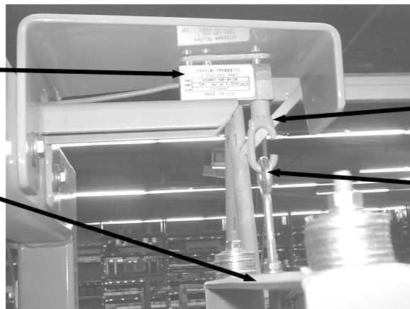
Figure 3-1. Hanging the Weigh Bucket Assembly From the Load Cell
