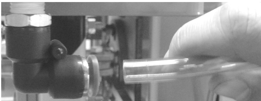
Figure 7-8. Inserting the Air Supply Line
