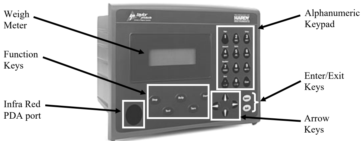
Figure 1. T3000 Control Panel
