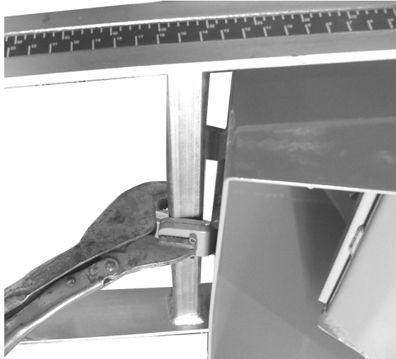
Figure 3-3. Clamping the Scale Beam Down
