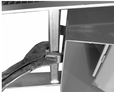
Figure 7-4. Clamping the Scale Beam in the Down Position
