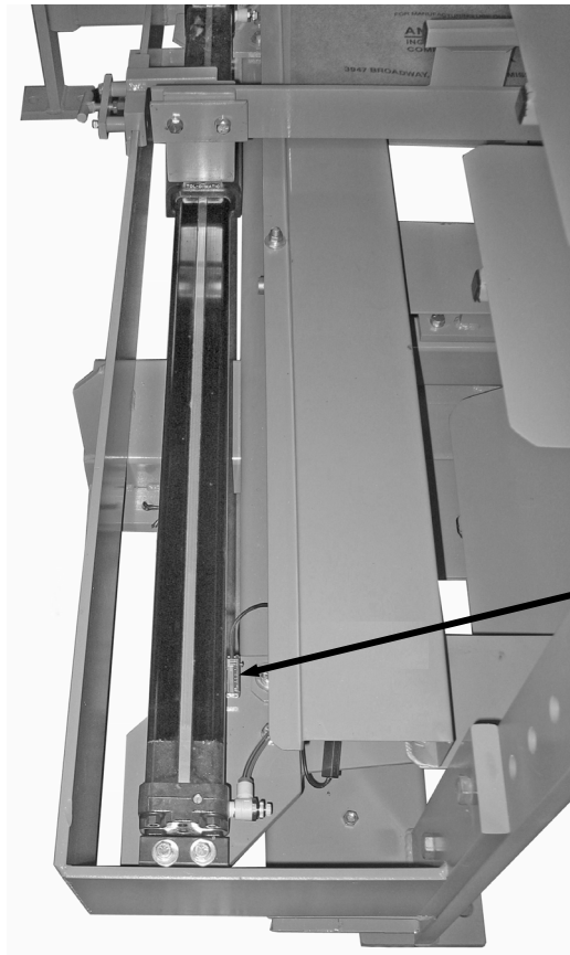
Figure 7. Bag Stack Pusher Home Proximity Switch (PR2)
