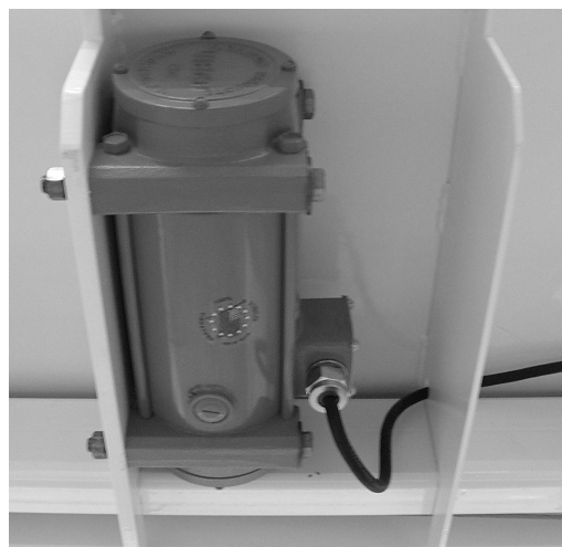
Figure 7-22. Electronic Vibratory Settler
