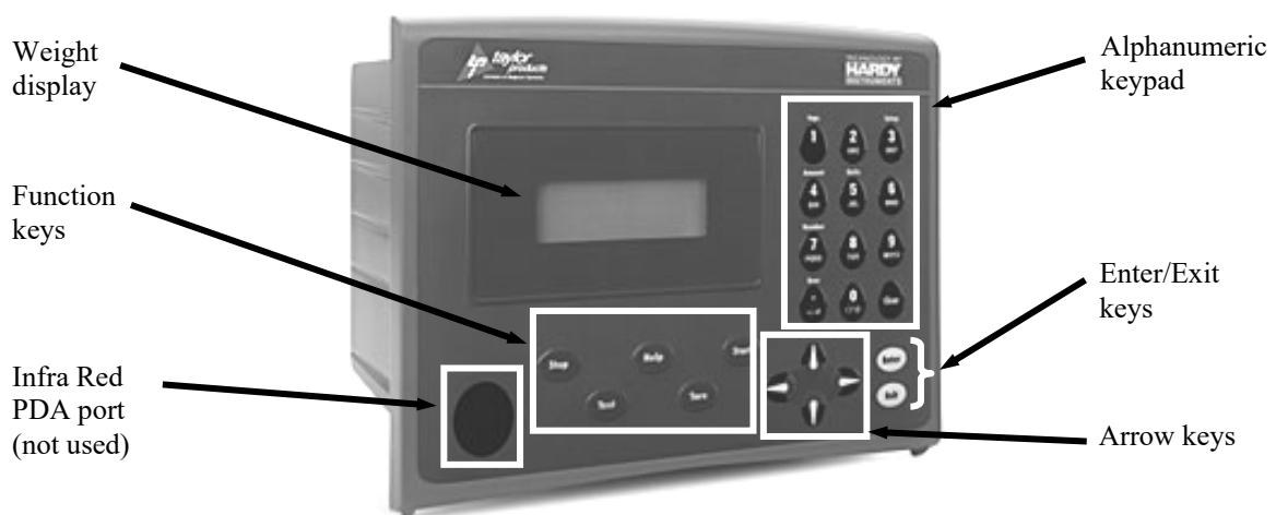
Figure 1-13. T3000 Control Panel
