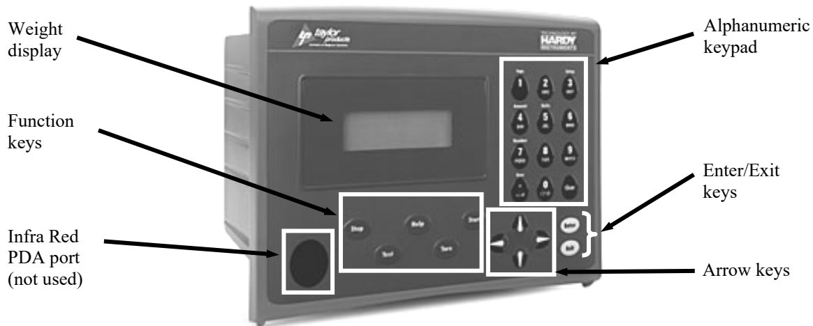
Figure 4-3. T3000 Control Panel
