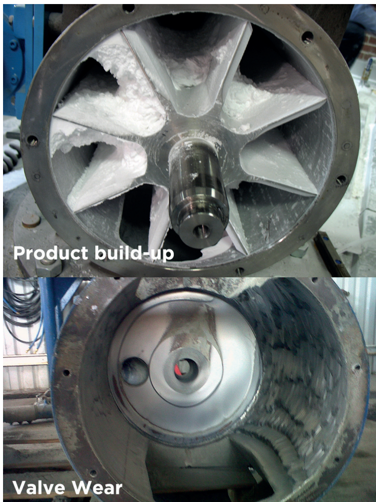
Image 4: Valve wear and product build-up
