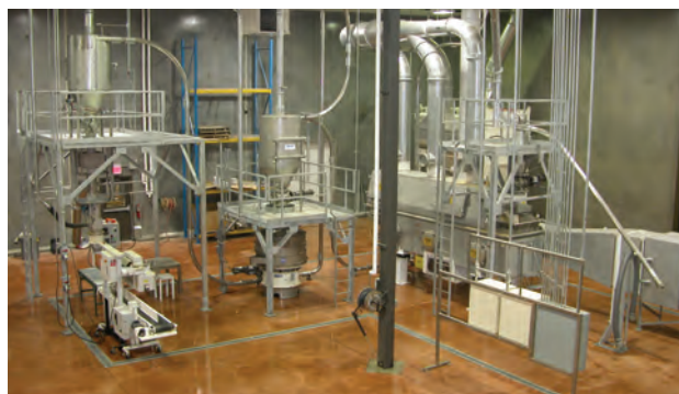
Pneumatic conveying system for food flavorings
