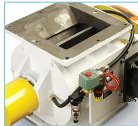
SAP uses high pressure plant air to prevent the conveyed material from coming in contact with the shaft seals, therefore extending the life of the seals.
