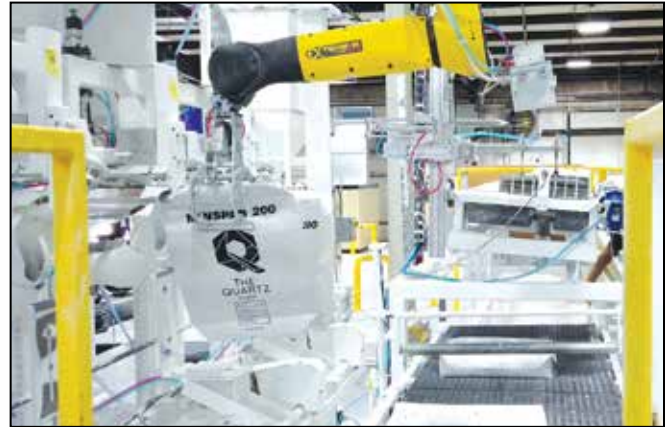
Model TRV-1000 robot placing 50 lb bags.
