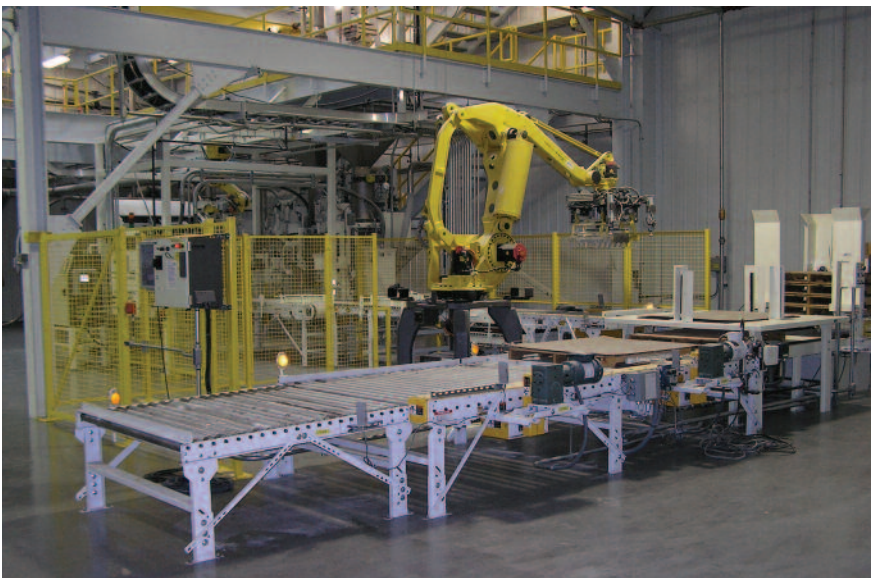
The automated palletizer’s four-axis robotic arm accurately stacks 50-pound bags on a pallet in a preset stacking pattern, ensuring safe transport to customers.
