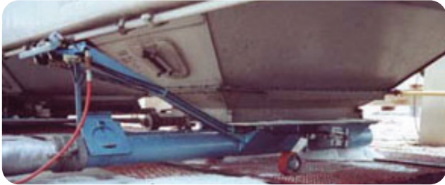
The innovative under-car adapter allows speedy vacuum unloading of railcars at the customer's delivery point.
